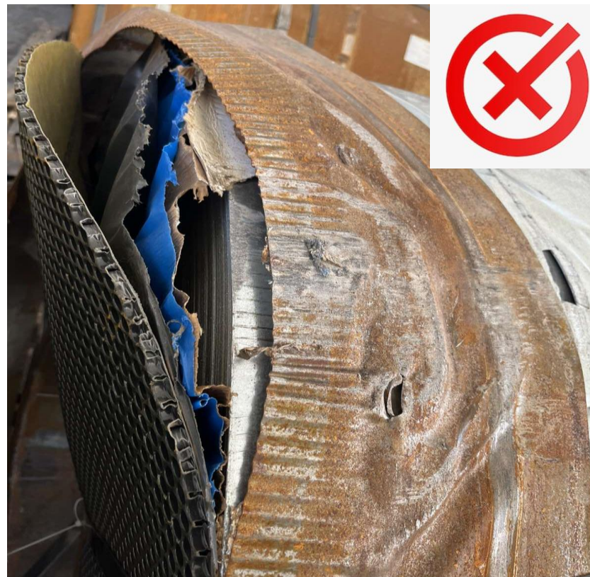
Displacement of the outer ring, exposing the rolled product
