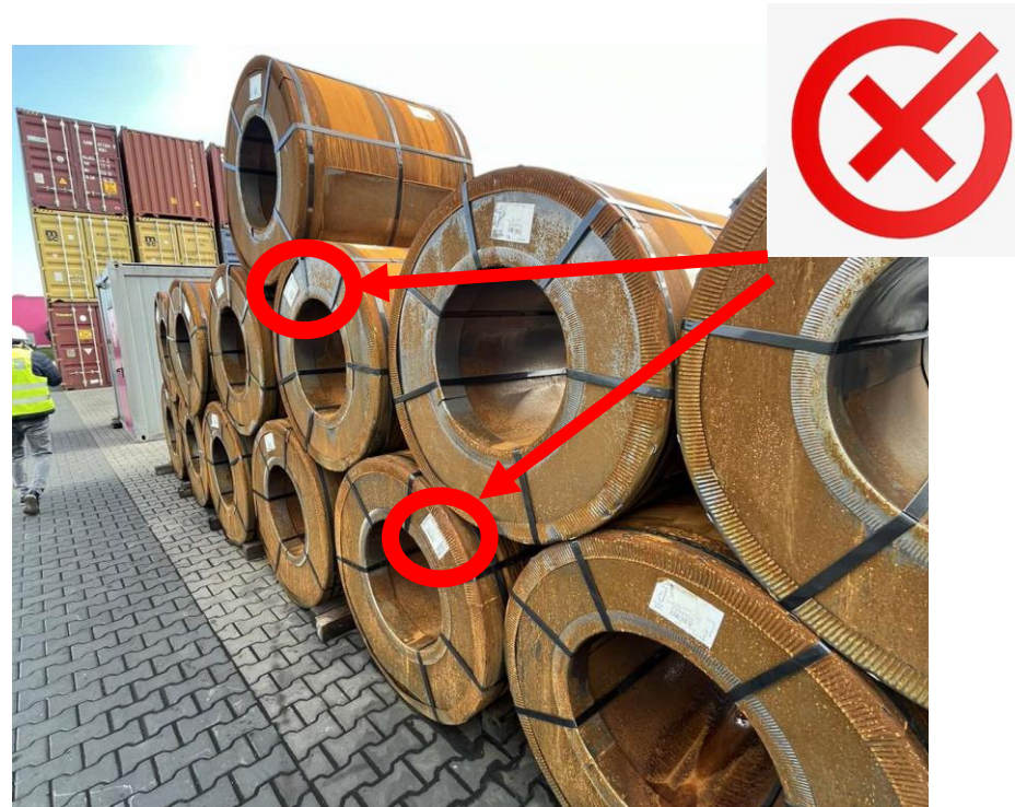
Wrong positioning of a coil, displacement of the coil top
